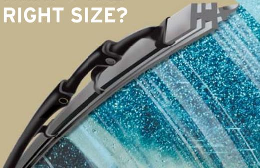
When replacing the blade, it's important you use the proper size specified for the vehicle. This helps ensure blades will clean the entire windshield area. Mounting the proper size blade on the correct arm is essential to prevent damage. The right wiper blade is often a different size than the left. Your Service Advisor knows your vehicle best and will recommend the right part at the right time.
